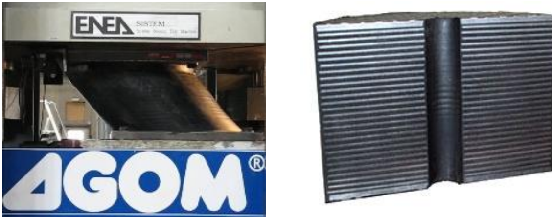
Figure 19: Typical round base isolator under lateral deformation (above-left). Cross section of a lead-core rubber base isolator (above-right). Images courtesy of AGOM Metal Rubber Engineering ( http://www.agom.it/ )
